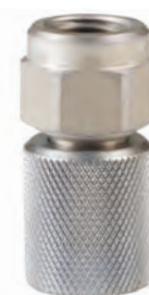
SMD20-1/4NPT-C6F Adaptor for process connection 1/4NPT (N04) on test coupling STAUFF Test 20 (connection thread M16 x 2)
