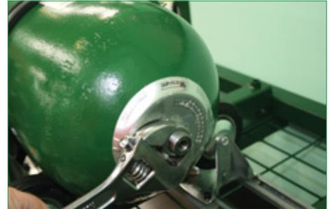
3. Fit Name Plate and Locknut to Bladder Stem.
