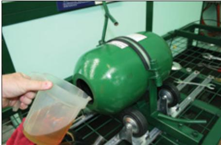
1. Ensure that the inside of the Shell is well lubricated with System Fluid.
