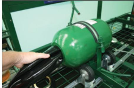
2. Take Bladder and remove Gas Valve. Remove all air from the Bladder and fold neatly. Position Bladder inside Accumulator so that the Bladder Stem protrudes through the small opening at the other end of the Shell.
