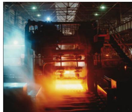
**Descaling of steel sheets and profiles.**
