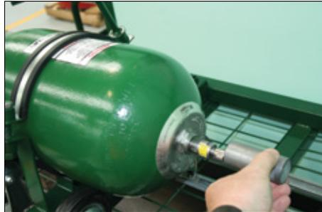
14. Fit the Gas Valve Protection Cap.
