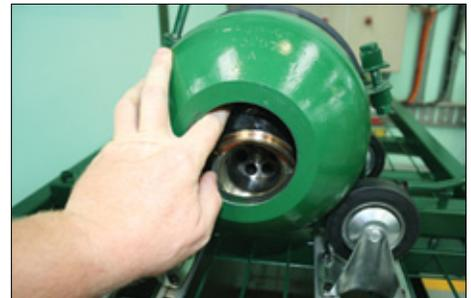
6. Slide the Anti-Extrusion Ring over the Fluid Port inside the Accumulator Shell.
