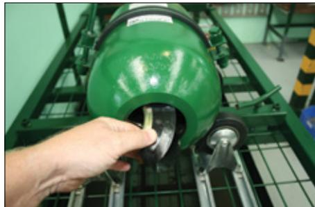
5. Place Anti-Extrusion Ring inside the Shell and make sure the metal ring is facing you.
