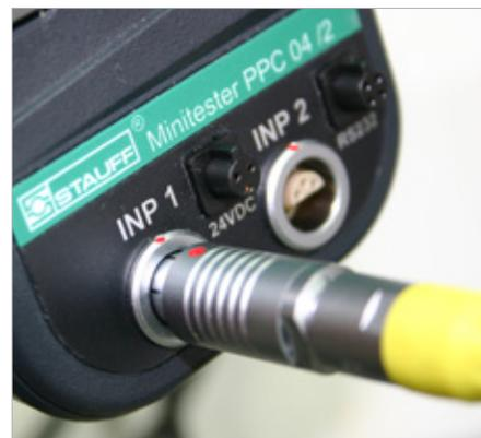
Two separate test inputs
