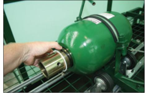
9. Remove the Nylon Back-up Washer along with the O-Ring.
