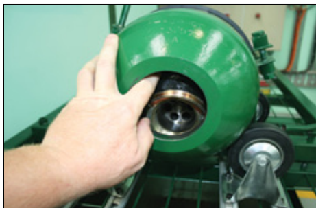
10a. Remove the Fluid Port Assy by first pushing the Fluid Port back into the inside of the shell.
