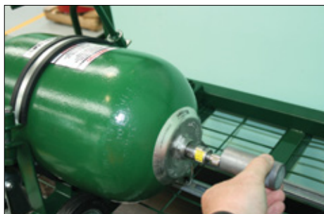
1. Remove the Protection Cap.
