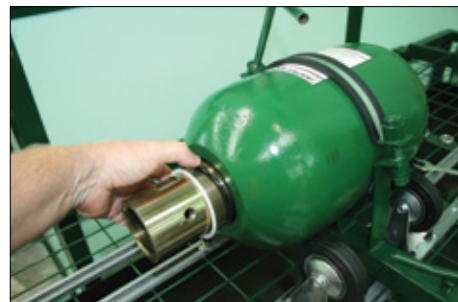
9. Remove the Nylon Back-up Washer along with the O-Ring.
