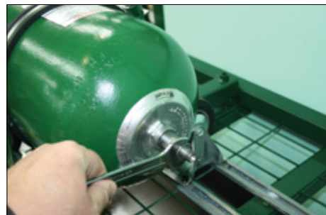
12. Fit the Gas Valve Assembly to the Bladder Stem and tighten to the correct setting. Ensure that when tightened the Bladder stem does not rotate.
