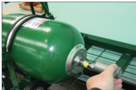
14. Fit the Gas Valve Protection Cap.
