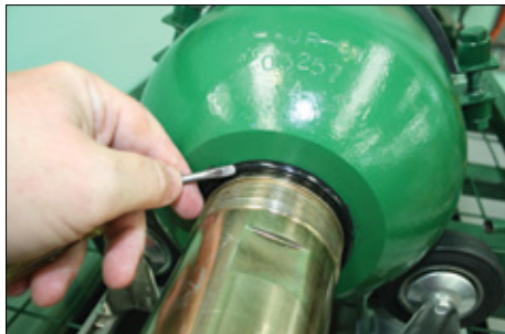
8. Holding the Fluid Port Body firmly install the O-Ring. Ensure no sharp tools are used and that the O-Ring is inserted evenly around the Fluid Port Body.
