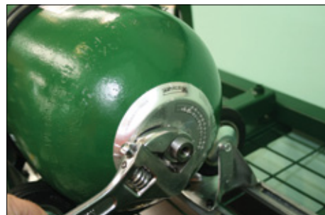
6. Remove the Bladder Lock Nut and Name Plate.
