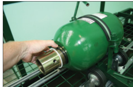
9. Ensuring the Fluid Port Body does not get dislodged - insert the Nylon Back-Up washer so that the rounded face on the washer faces the O-Ring.
