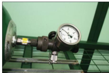
3. Attach STAUFF pre-charging head and release any pre-charge from the Accumulator.
