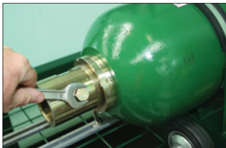
7. Remove the Bleed Valve on the Fluid Port.
