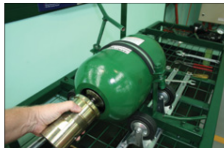
10c. The Fluid Port can then be removed from the shell.
