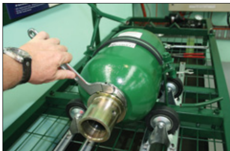
10. Attach first the Flanged washer and then the Lock-Nut. Ensure the Lock-Nut is tightened using an appropriate spanner.
