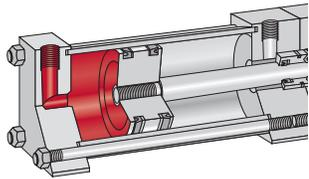
1. Low pressure air is applied to the large surface piston during the entire work stroke. The input pressure of BA Boosters is rated at 250 PSI air.
