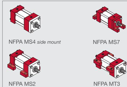
The side or lug mounted cylinder provides a fairly rigid mount. This type of mount can tolerate a slight amount of misalignment when the cylinder is fully extended, but as the piston moves toward the blind end, the tolerance for misalignment decreases. It is important to note that if the cylinder is used properly (without misalignment), the mounting bolts are either in simple shear or tension without compound stresses.
