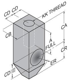
**NOTE:** The Rod Clevis and Rod Eyes are designed for use with the standard *Milwaukee Cylinder* Style No. 2 Rod End. When ordering these accessories, be sure to match the thread size of the Style No. 2 Rod End of the rod size you ordered to the thread size of the accessory you require.
