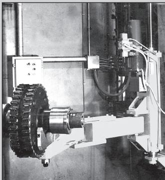
Large and complex cutters are often impossible to handle without some mechanical assistance. The Pow'r Arm™ was adapted for this specific application.
