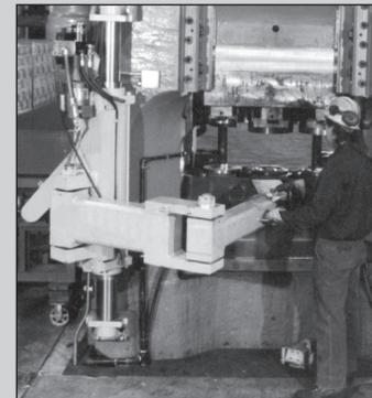
Large shear blades are used to cut steel bars and billets. When these blades become worn the Pow'r Arm™ performs speedy removal and replacement of the blades safely with minimal disruption to the process.
