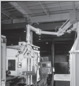
Parts are selected from pallets and moved to working stations. The smooth, positive hydraulic control of the Pow'r Reach™ permits picking and positioning of expensive parts safely and precisely.
