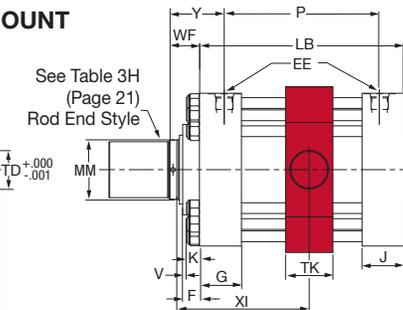
**TABLE 1H** The dimensions given on this table are affected by the piston rod diameter and the stroke.
