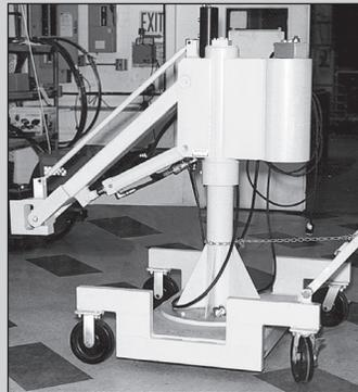
Portable dolly-mounted Pow'r Reach™ provides flexibility to accommodate a wide variety of applications. For stability, a counterweight is welded to the column of these models.
