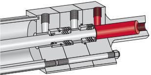
3. When the ram enters the high pressure seal, it immediately boosts the hydraulic pressure up to the rated value. Because of the extra ram seal assembly, the output pressure of this model is limited to 3,000 PSI.
