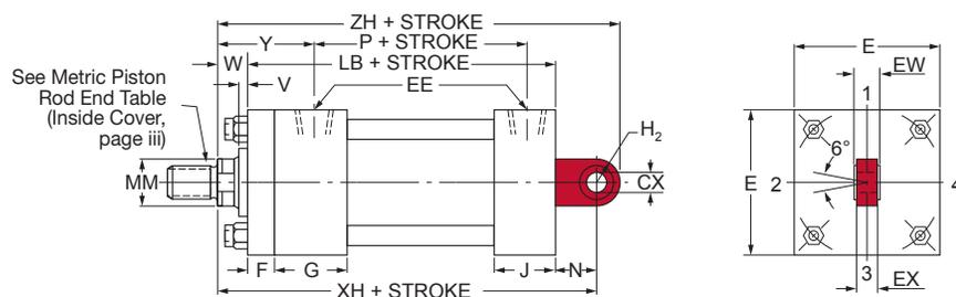
**TABLE 1MH** The dimensions given on this table are affected by the piston rod diameter and the stroke.
