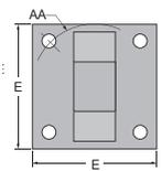
\* Eye Bracket only. Eye Brackets with suffix letter "A" reflect revised NFPA standards for F and FL dimensions.
