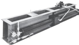
A Milwaukee Cylinder designed special booster featuring a 10" bore, 60" stroke and a 5½" rod. This booster, mounted on the side of a steel "I" beam, converts a 3,000 psi oil input to an 8,000 PSI output of an ethylene-glycol solution with a total high pressure displacement of 1,400 cubic inches. The booster also had to be designed to operate over a temperature range from -65° to +100° F.
