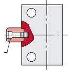
Removable trunnion pins are available on models A71 and A72. They can be used on all bore and rod combinations, except on the largest oversize rods offered
