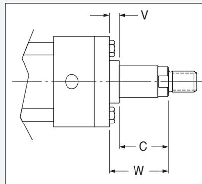
**To Compute:**  $W = (\text{Stroke} \times \text{Min. Length Factor}) + 1\frac{3}{8}"$
