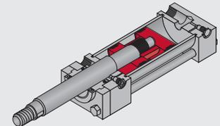
The second stop tube design is the double piston stop tube. This stop tube is primarily used for cushion rod end air cylinders. Unlike the single piston stop tube design, the double piston stop tube provides additional strength for excessive side loading and adds additional bearing area to the cylinder.
