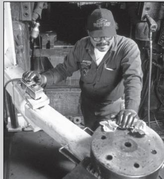
In automated forging processes, hot metal blanks are fed automatically into a progressive die. Each die segment may weigh several hundred pounds and must be handled quickly, easily and safely.
