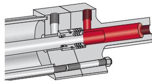
3. Oil flows out, and back in, the same port on the high pressure end of the BD booster. Make up oil is provided through an external check valve or needle valve.
