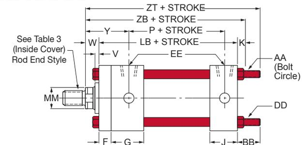
**TABLE 1LH** The dimensions given on this table are affected by the piston rod diameter and the stroke.
