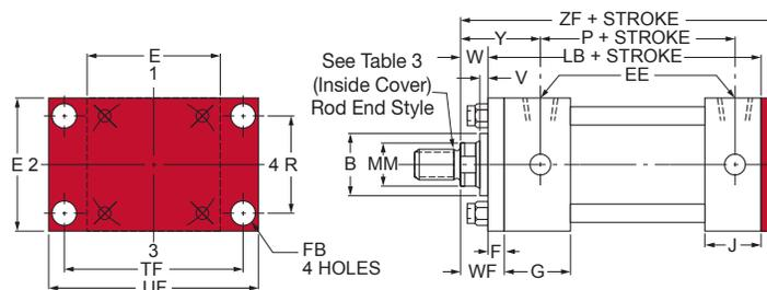
**TABLE 1LH** The dimensions given on this table are affected by the piston rod diameter and the stroke.
