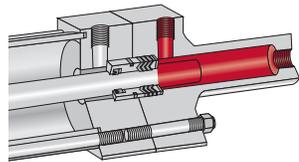
2. The rod of the BD booster is constantly under high pressure throughout the entire work stroke. It has but a single seal assembly.
