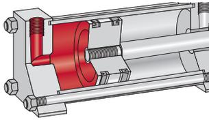
1. Low pressure air is applied to the large surface piston during the entire work stroke. The input pressure of BD Boosters is rated at 250 PSI air.
