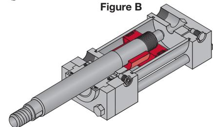
The stop tube is located between the piston and the rod end cap. It limits the extended stroke of the cylinder, providing additional strength for less cost and reduced weight than the use of an oversize rod.
