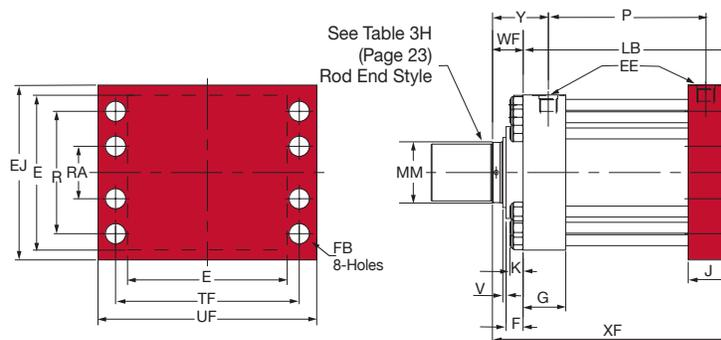
**▼ TABLE 1H** The dimensions given on this table are affected by the piston rod diameter and the stroke. (H21, H22)
