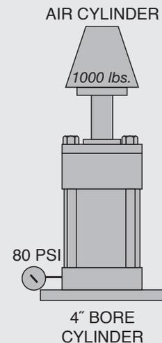
The exact speed of an air cylinder cannot be calculated. Air cylinder sizing depends on the degree of overpowering to move the load, valving, piping, and other factors which usually are unknown and cannot be measured. For further information on air cylinder sizing and speed, refer to page 100.
