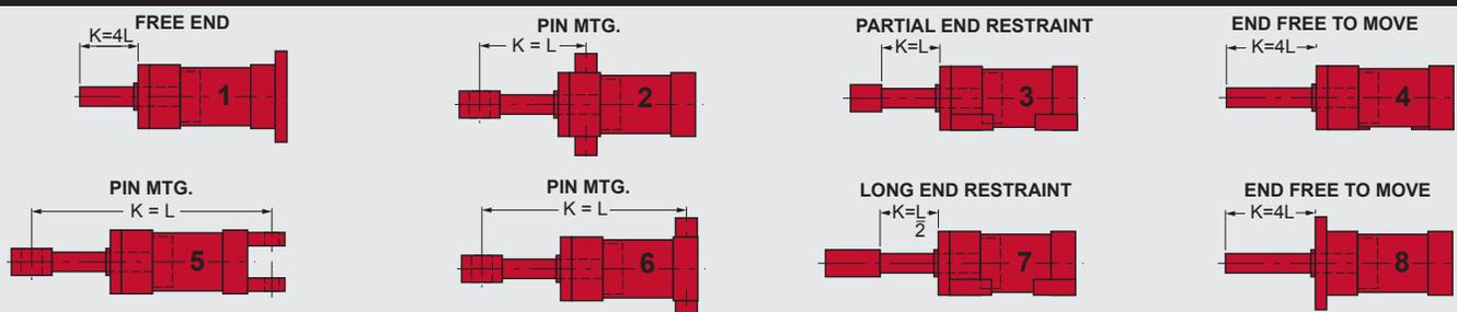
When mounting long stroke cylinders, care should be taken to assure cylinder alignment over the entire length of stroke. The use of external guides or swivel bushings is recommended to reduce side load conditions and prolong the cylinder's service life.
