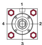
Ports are located in position #1 as standard unless otherwise specified. By using the position numbers given with the end views in the dimensional data section of this catalog, ports can be arranged in any one of four 90° positions in relation to the cylinder mounting. When ports are relocated on a cushioned cylinder, the cushion needle and ball check are automatically relocated to hold their relationship to the port as on a standard cylinder, unless otherwise specified at the time of the order.
