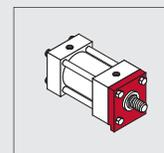
The key mount retainer plate is a mounting option designed to add stability to foot and side mounted cylinders. The retainer plate is extended below the mounting surface of the cylinder. This extension may be fit into a milled keyway, eliminating the need for welded keys or locator pins.
