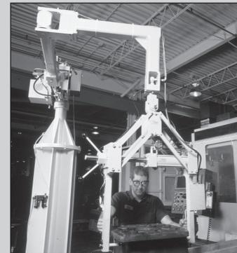
A Pow'r Reach™ is used to position parts in machining centers. It is useful and effective because of the ease and convenience with which the heavy parts are handled.
