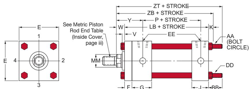
▼ **TABLE 1MH** The dimensions given on this table are affected by the piston rod diameter and the stroke.
