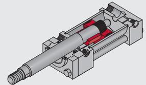
At *Milwaukee Cylinder*, we offer two stop tube designs. The single piston stop tube design is common to all cylinders except cushion rod end air cylinders. A stop tube will increase the overall length of the cylinder and will alter the mounting dimensions on most models by the length of the stop tube.
