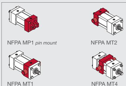
All pin and trunnion mounted cylinders need a provision on both ends for pivoting. This type of mounting is designed to carry shear loads and requires that the trunnion or pivot pins are rigidly held by closely fit bearings for the entire pin length.
