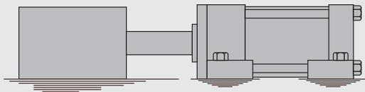
Cylinders perform a wide variety of applications and are often used in place of larger, more expensive mechanical systems. One such application is when a cylinder is used to move a high friction sliding load. Some examples of this are: machine slides, pallet shuttle systems on automated machinery, milling machine tables, and grinder tables.
