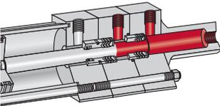
2. The rod advances through hydraulic fluid that is not yet contained under pressure. The rod is traveling under the same pressure as the air supply.
