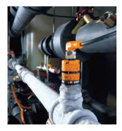
The compact TK Series temperature switch and its integrated 316 stainless steel RTD probe measure only 4" long and can be directly mounted into a pipe.
