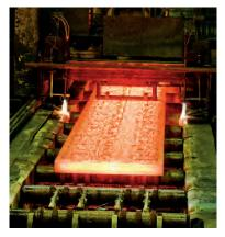
The TW Series temperature sensor can be used to detect a hot steel slab by measuring the infrared radiation intensity emitted from the hot slab.
