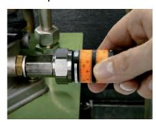
TK temperature switches feature mechanical adjustment dials that rotate to quickly establish the setpoint and resetpoint.
