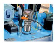
The TD temperature transmitter reliably monitors the fluid temperature in many industrial applications.
