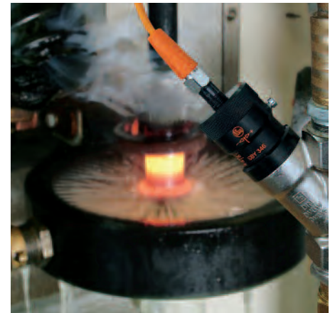
The mechatronic sensor reliably monitors the flow of water in cooling loops of an induction furnace.
