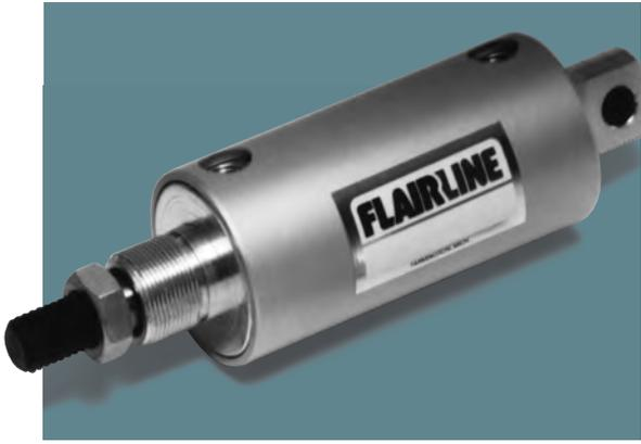
DI type cylinders expand Flairline's I type cylinders by offering double U-cup pistons with wear strips and bronze rod bearings for use when side load conditions are present. External dimensions may be interchanged with competitors to minimize expensive inventory or engineering changeovers.
