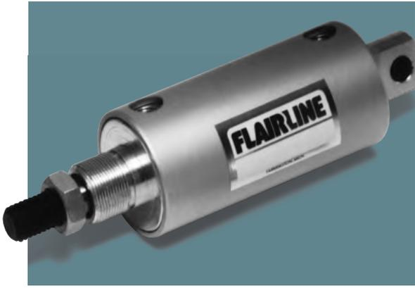
DSI type cylinders expand Flairline's SI type cylinders by offering double U-cup pistons with wear strips and bronze rod bearings for use when side load conditions are present. External dimensions may be interchanged with competitors to minimize expensive inventory or engineering changeovers.
