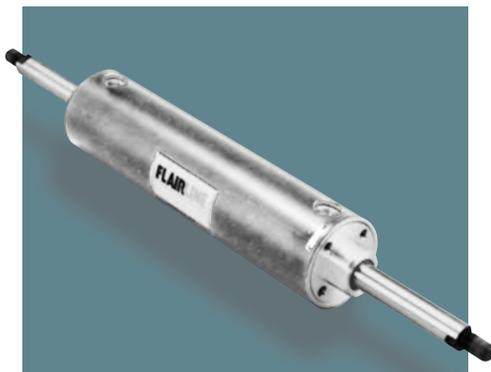
Flairline double-acting double-ended NFPA interchangeable cylinders feature piston rod extensions from each end and a choice of F or O type pistons. As one end is extended, the opposite end is retracted. Working range (stroke), force and speed are equal in both directions so work can be accomplished at both ends simultaneously. See page 23 for dimensional data, pages 24 and 25 for mounting styles, page 25 for rod end styles and page 26 for accessories. For special options, see page 28.
