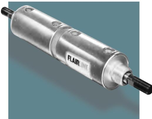
Cap-to-Cap models consist of two F, O, H or D type cylinders joined at the cap end by a common center section. Each unit can be operated independently of the other to accurately attain and repeat three positions when both units are the same stroke and four positions when each unit is a different stroke. See page 7 for dimensional data and page 10 for mounting accessories. For special options, see page 16.
