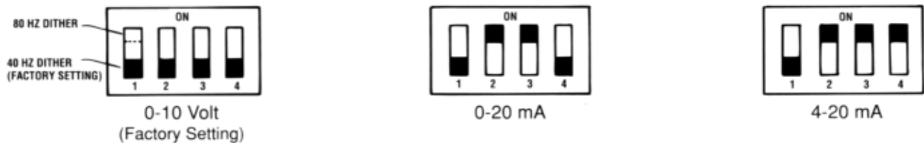
Figure 10. DIP Switch Settings for Dither and Input Signal
