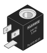
Standard coils fit all general purpose solenoid valves, except ISO valves with CNOMO air pilots. Coils are encapsulated to keep out water, oil and other contaminants providing splash proof protection when used with sockets below. The 3-prong plug includes a ground connection for the coil frame. Terminals can also be connected using crimp-on wire terminals with a ¼" spade dimension. Coil power consumption: AC (60Hz) is 3.5VA, DC is 2.5 W.
