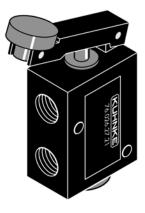
Can be used as end of travel device or thumb valve. Lever travel is 3/8" (10mm). Actuation force is 4.5 Lbs.
